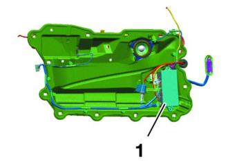
The output for the ZV drives is controlled by internal final stages.
